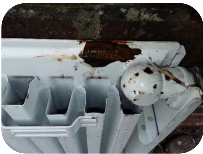
Rusty old radiator
